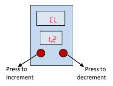
Press both buttons together to save the changes. The unit returns to its normal display after saving the new current limit.
