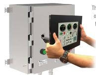
The EZTouch Series 7 HMI features online editing and a two-part assembly that allows the display and touch-screen to be easily replaced without disturbing the logic and communications electronics.
